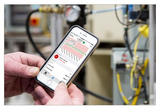
**Voice of the Machine Mobile App** gives access to machine and process measurements right on your mobile device. The user-friendly interface makes connecting to sensors uncomplicated and measurements easy-to-read. With customizable dashboards and alarms, you can focus on the data that's most important to you and be alerted when your measurement thresholds are exceeded. Exporting of data is done with a click of one button, which sends a .csv file right to your email.
